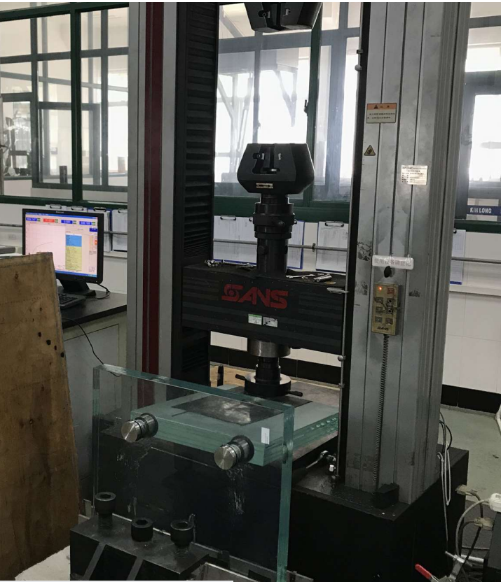
Glass Stair Joint Strength Test
