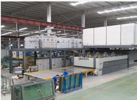
2440*5000mm Imported Tamer Tempering Furnace
